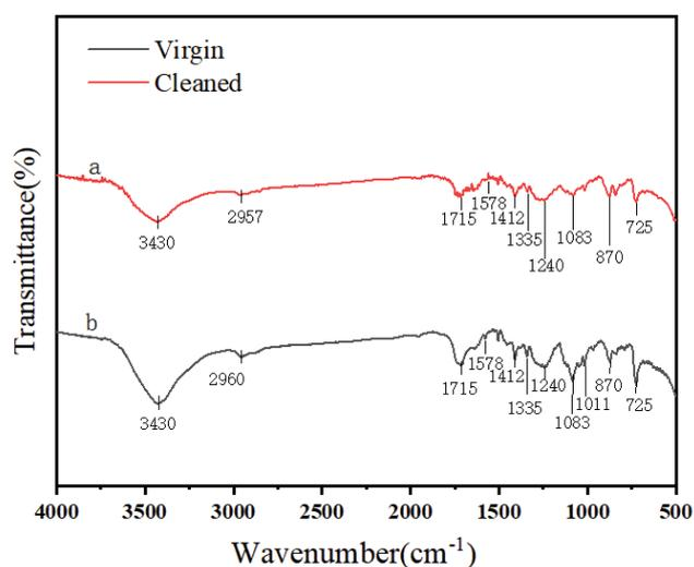
Fig. 6. Fourier-transform infrared spectra of virgin membrane (a), and cleaned membranes (b).
