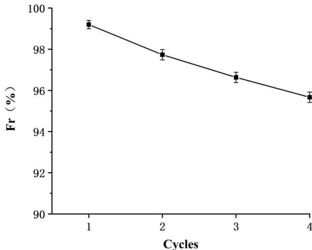
Fig. 8. Membrane flux recovery rate of polyethersulfone composite membranes in SAOPW filtration experiments.
