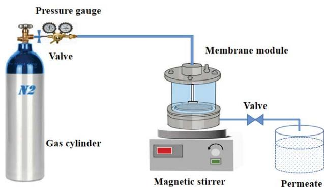
Fig. 1. Schematic of the ultrafiltration set-up.
