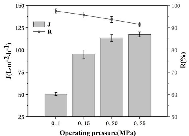
Fig. 2. Effect of the operating pressure on the permeate flux and oil removal rate.
