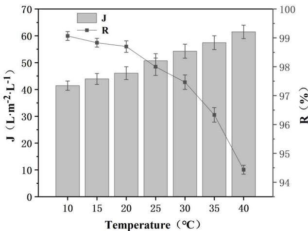
Fig. 3. Effect of the feed temperature on the permeate flux and oil removal rate.
