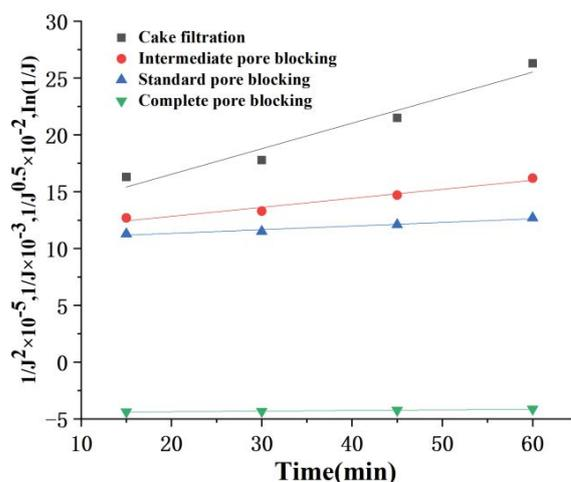
Fig. 10. Plots of flux functions vs. time for four different pore blocking models.
