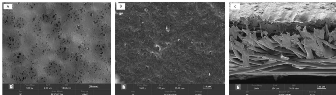
Fig. 5. Scanning electron microscopy images of polyethersulfone composite membrane: (A) virgin membrane surface, (B) fouled membrane surface, and (C) cross-section.
