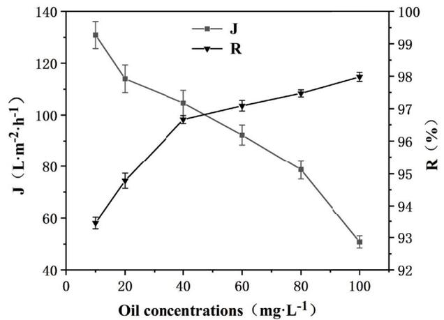
Fig. 4. Effect of the feed concentration on the permeate flux and oil removal rate.
