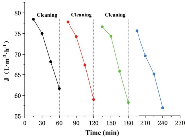
Fig. 7. Flux decline behaviors of polyethersulfone composite membrane with different filtration cycles.
